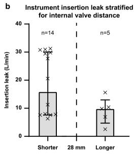
**Fig. 5** a Leak during instrument insertion trocars grouped per trocar size and used instrument size, median and inter-quartile range per group. **b** The effect of valve distance compared to the tool tip length of the surgical instrument, in this case longer or shorter than 28 mm. The height of the boxes is the median value, the whiskers represent the inter-quartile range and the crosses are each individual trocar
