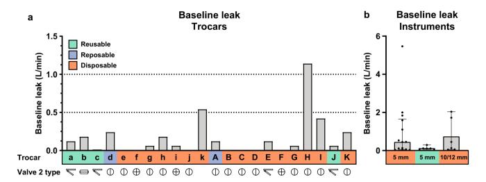
**Fig. 3** a Baseline flow measurements in trocars at 15 mm Hg. Along the x-axis the trocar names are noted, the colours correspond to the trocar type. The type of valve 2 is denoted by a symbol under the result of each trocar and is detailed in Table 1. As trocar k had
