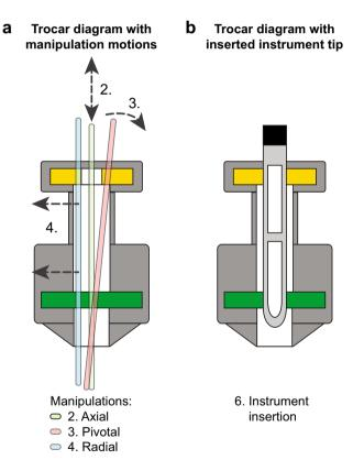
**Fig. 2** a Manipulations of the rod within the trocar, in axial (2), pivotal (3) and radial (4) directions. Axial manipulation oscillation are performed with a 5 cm amplitude. During the pivotal and radial manipulation the rod is maximally displaced. **b** During the instrument insertion test, a grasper with a fenestrated structure was inserted into the trocar and kept in contact with both valves to allow for an open passage of gas
